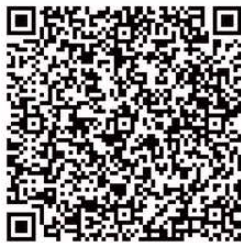
Version 10 (57×57). Content: "VERSION 10 QR CODE, UP TO 174 CHAR AT H LEVEL, WITH 57X57 MODULES AND PLENTY OF ERROR CORRECTION TO GO AROUND. NOTE THAT THERE ARE ADDITIONAL TRACKING BOXES"
