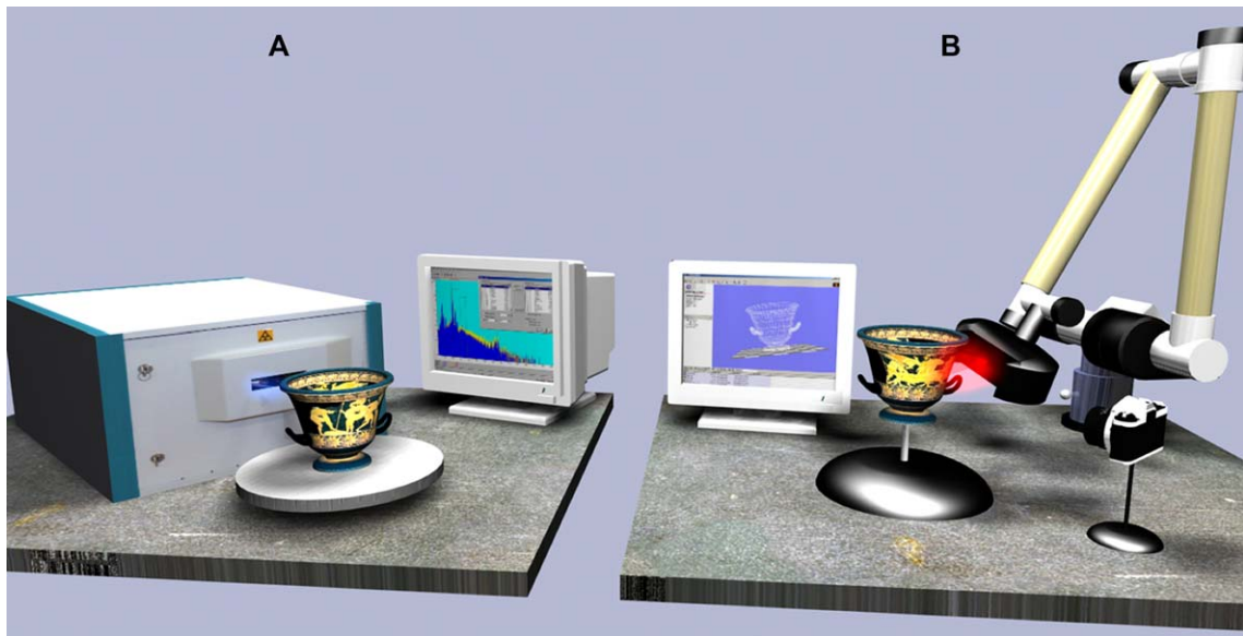
Fig. 1. Representation, at work, of technologies that provide with surface and geometry data; (A) 3D laser scanner for surface geometry (0.1 mm resolution), (B) point chemical composition with a \mu -XRF system (0.1 mm resolution).
